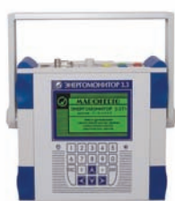
Energomonitor 3.3T1 (Reference instrument for testing energy meters of accuracy classes up to 0.5S)
