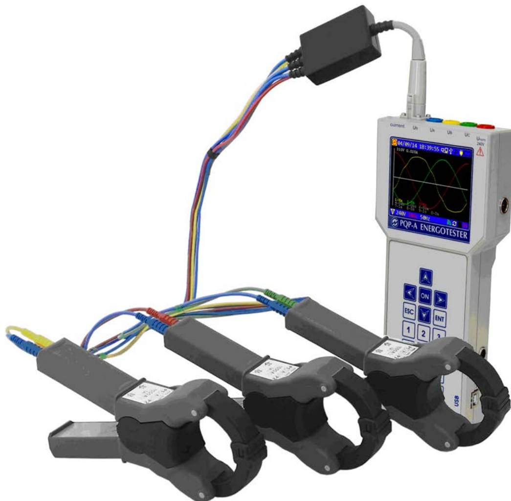
Fig. A3 Connecting PQP-A Energotester to 1000A Current Clamps
