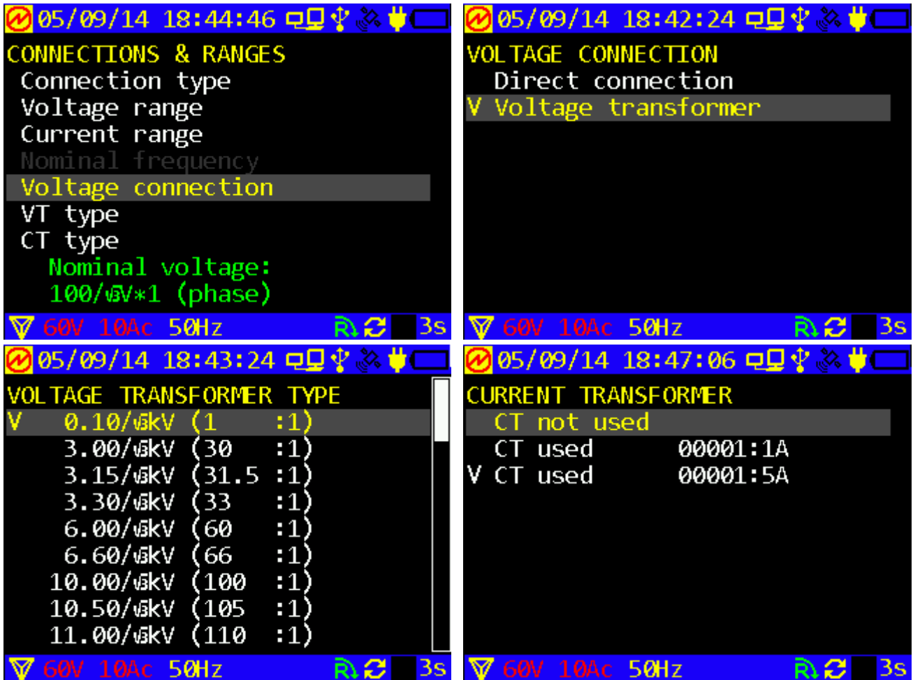
Fig. 4.4.4 Transformer selection windows
