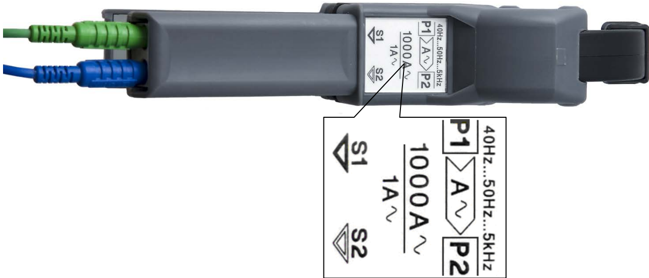
Fig. A4 Stenciled marks "source → load" on a 1000A Current Clamp
