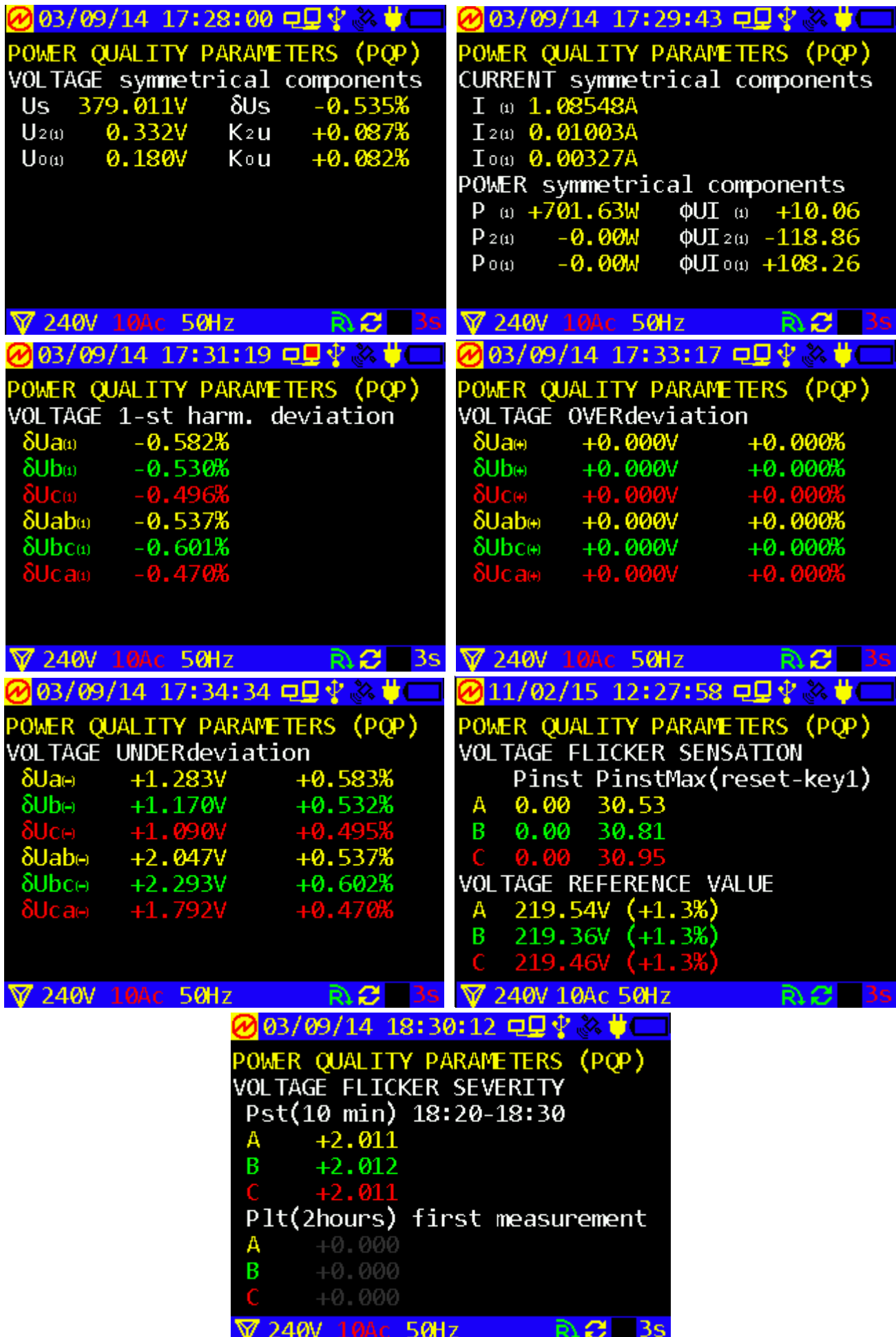
Fig. 4.2.4 View of PQP screens
