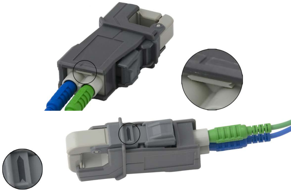
Fig. A2 Flow direction mark 'source → load' on the 10A and 100A clamps
