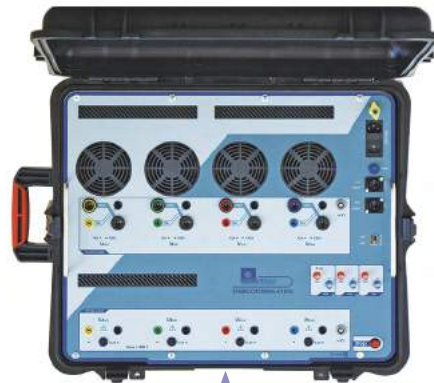
Phantom power and test signal source Energoforma- 61850
